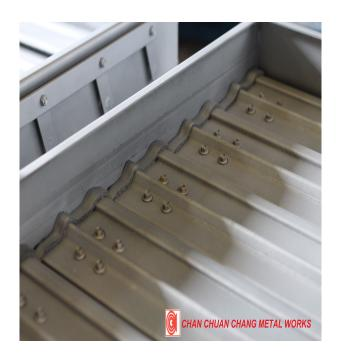
All openings such as sides, tops, bottoms & middle of blades are sealed with Gasket Forms to prevent excessive leakage through the dampers. The Gasket Form Seals are able to withstand between -57°C to 125°C.
